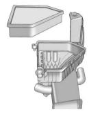
8. Remove the air cleaner filter from the air cleaner housing.
